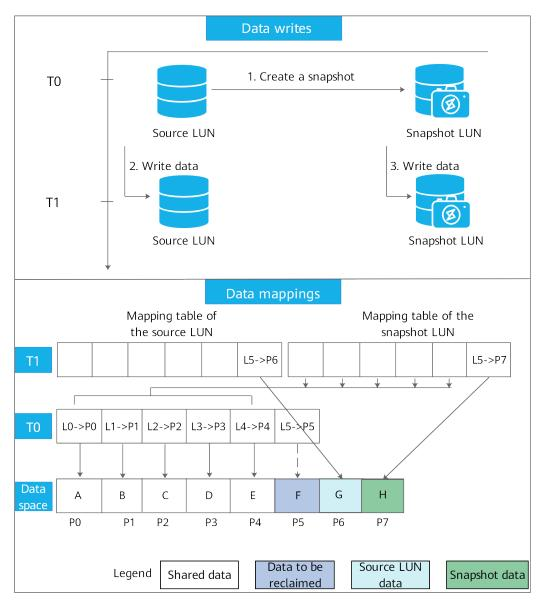
Figure 6-2 Reading and writing a snapshot
