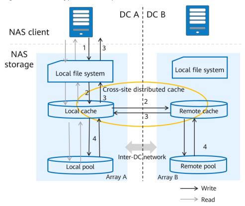
Figure 6-14 NAS HyperMetro I/O process
