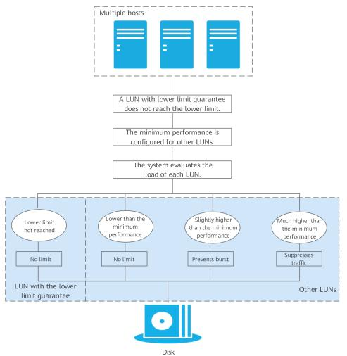
Latency assurance is to prioritize requests of objects that have latency objectives. If latency assurance is not achieved, the latency objectives are converted into traffic control objectives and guaranteed in the same way as lower limits.
