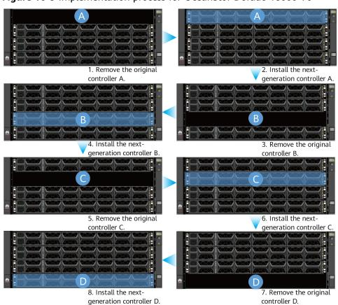
Figure 10-9 Implementation process for OceanStor Dorado 18000 V6
