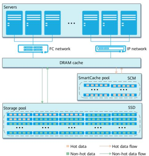
Figure 5-15 SmartCache working principles
