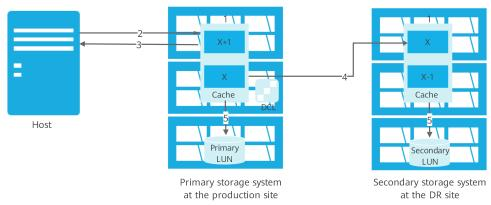
Figure 6-12 Working principles of HyperReplication/A
