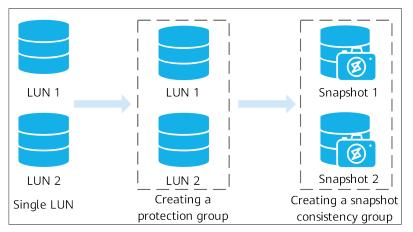
Figure 6-4 Working principles of the snapshot consistency group
