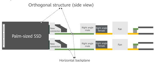
**Figure 3-31** Orthogonal connection structure of the horizontal backplane (side view)
