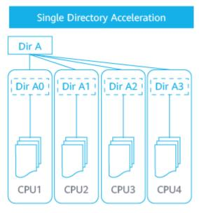
When a directory and its files are frequently accessed, OceanStor Dorado distributes the load of this directory to multiple cores of multiple CPUs for parallel processing and improved efficiency.
