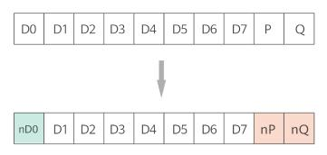
Figure 4-14 Write amplification of traditional RAID 6
