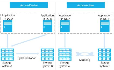
Figure 6-17 Active-passive and active-active storage architectures
