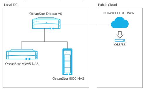
Figure 7-2 Typical CloudBackup networking
