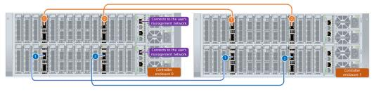
Figure 3-47 Direct connections for scale-out to eight controllers
