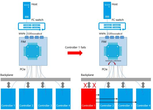
Figure 3-45 Service failover between controllers
