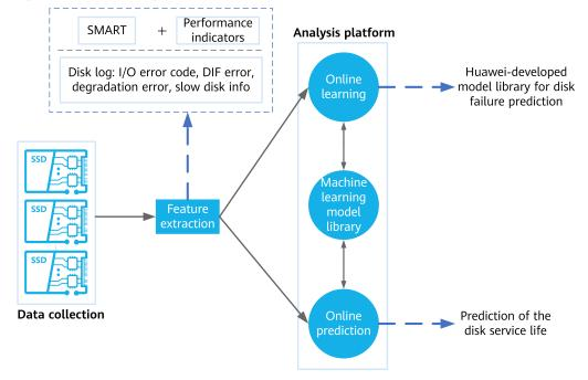
Figure 12-7 Working principles of disk health prediction
