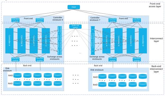
Figure 3-41 Interconnection of 32 controllers
