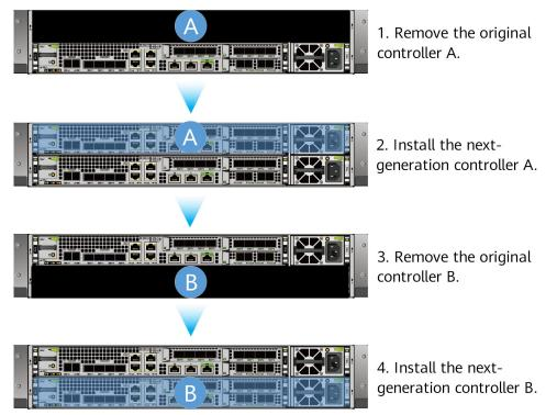
Figure 10-7 Implementation process for OceanStor Dorado 3000 V6
