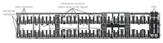
Figure 3-33 Air flow on the horizontal backplane
