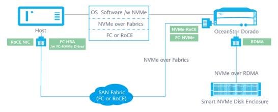
FC-NVMe applications can be carried by the existing FC SANs and switches of data centers. Customers only need to install the NVMe driver on the FC HBAs of the hosts to support NVMe, protecting the original investment.
