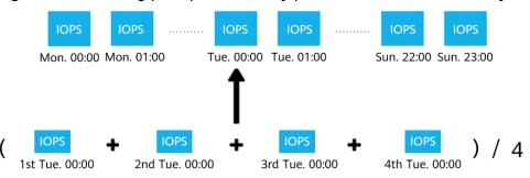
**Figure 12-9** Working principles of weekly performance fluctuation analysis
