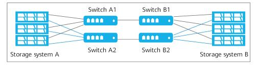
Figure 6-19 Fully interconnected network between storage systems
