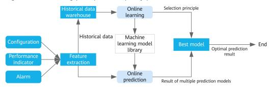
Figure 12-6 Working principles of capacity prediction
