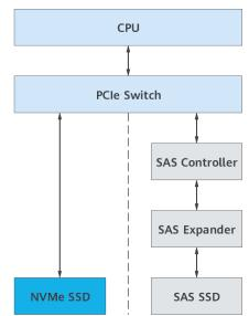
Figure 3-35 Transmission paths of NVMe and SAS SSDs
