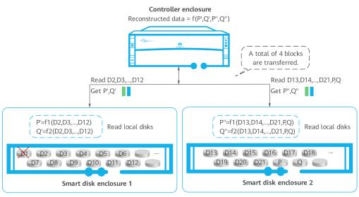
Reconstruction tasks are offloaded to smart disk enclosures, reducing the drop in system performance to less than 10% in the event of data reconstruction due to disk failures (system performance drops by 20% if traditional disk enclosures are used).
