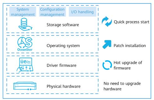
Figure 10-6 Component-based upgrade
