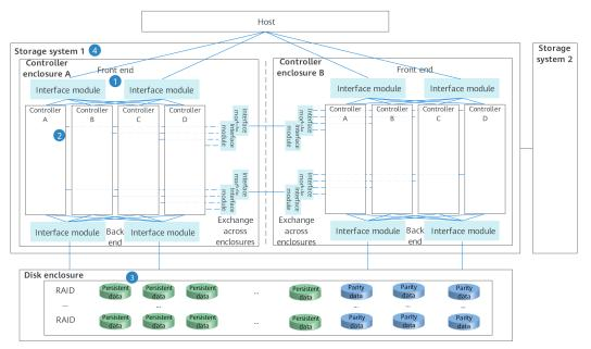
**Figure 8-6** Multi-layer redundancy and fault tolerance design (high-end)
