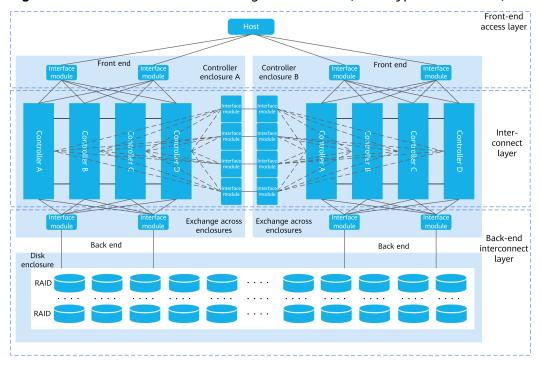
Figure 3-40 Full-interconnection of eight controllers (with HyperMetro-Inner)
