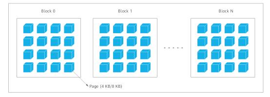
The multistreaming technology classifies data and stores different types of data in different blocks. There is a high probability that data of the same type is valid or garbage data at the same time. Therefore, this technology reduces the amount of data to be migrated during block erasure and minimizes write amplification on SSDs, improving the performance and service life of SSDs.
