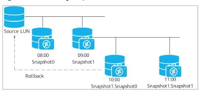
Figure 6-3 Cascading snapshot and cross-level rollback
