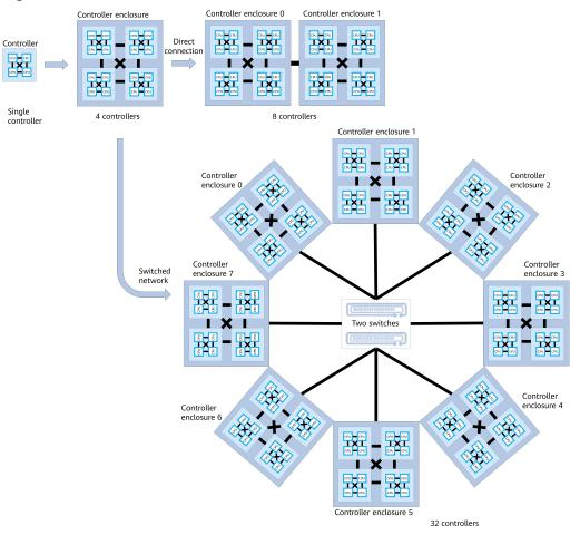
Figure 3-39 Full-mesh balanced hardware architecture (direct connection)
