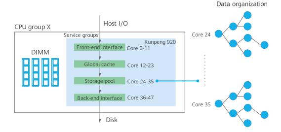
Figure 4-12 Lock-free design between CPU cores
