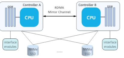
**Figure 3-11** Logical architecture (1) of a mid-range storage system (with SAS SSDs)
