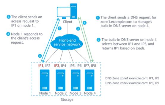
A host can use a domain name to access NAS services on a storage system. A domain name system (DNS) can balance the loads of multiple IP addresses for a domain name. Traditional external DNS servers have the following problems:
