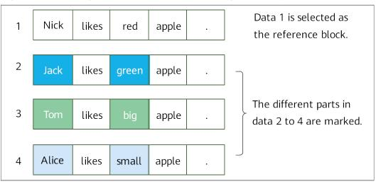
**Step 3** The system retains all content of the reference block. For the other data, only the different parts and their locations are recorded. **Figure 5-4** shows the deduplication result.
