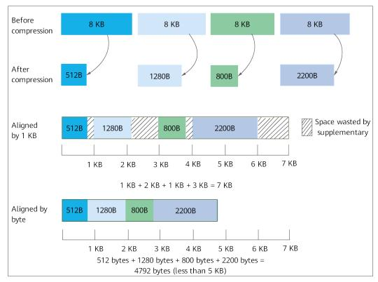
Figure 5-6 Alignment of compressed data by byte
