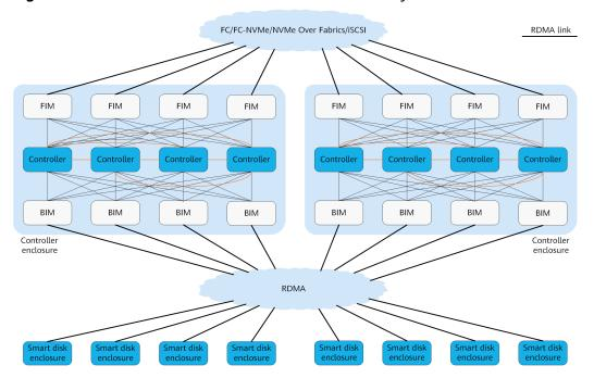
Figure 3-50 RDMA interconnection for an 8-controller system
