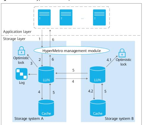
Figure 6-13 SAN HyperMetro write process
