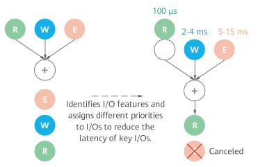
Figure 4-19 Read first on SSDs
