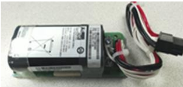
Figure 6 Battery Backup Unit
